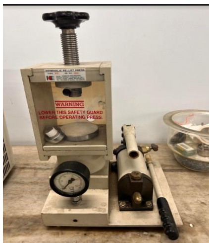
Hydraulic Press facility for making the pellets
